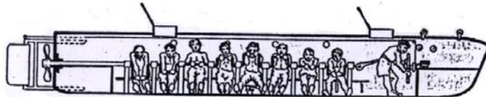
Sketch of how the C.S.S. Hunley operated by its nine man crew
